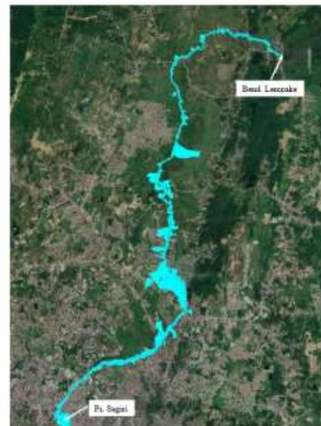
**Figure 14.** Mapping of Flood Inundation in the Remaining Basin with a Return Period of 5 Years (Scenario 2)
