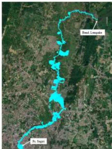
**Figure 13.** Mapping of Flood Inundation in the Remaining Basin with a Return Period of 5 Years (Scenario 1)
