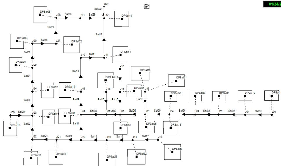
**Figure 6.** Modeling of Sub-Catchment Areas, Junctions, and Conduits in the Study Area.
