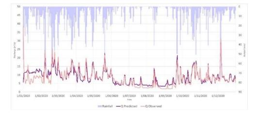
Fig 11. Hydrograph comparison of discharge data from model simulation results and observation discharge for one year in daily terms in 2020.
