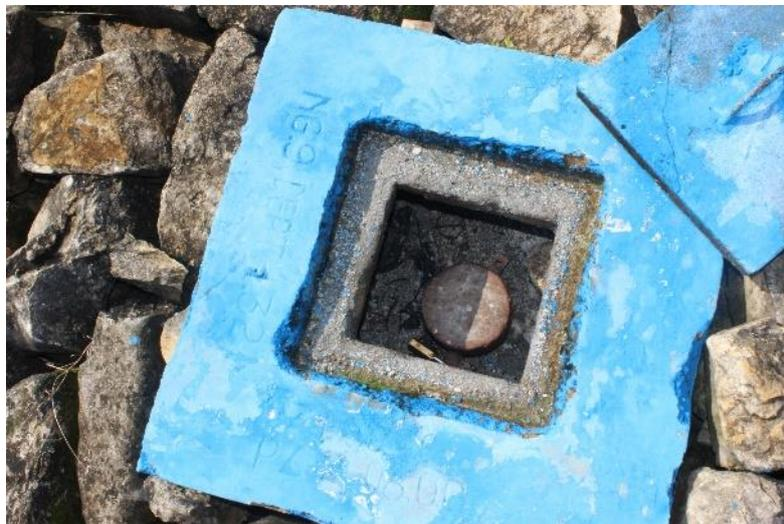
**Figure 2.** Inspection of stand pipe piezometer at Ngancar Dam
