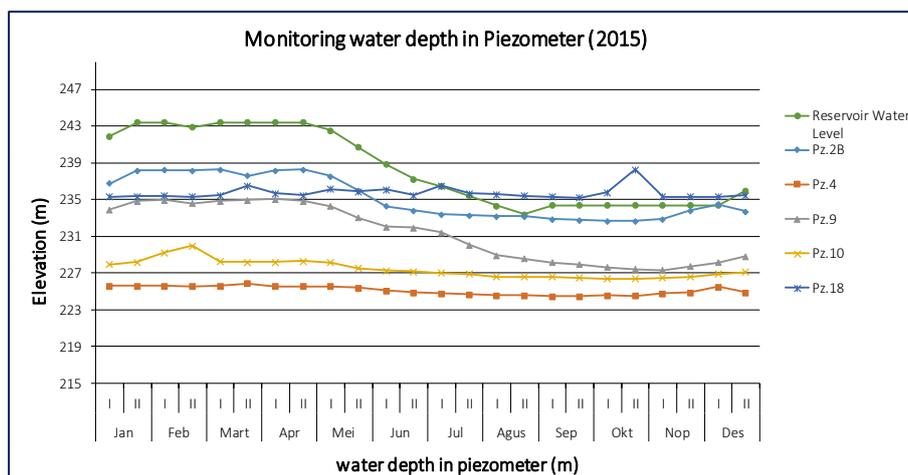
**Figure 4.** Change the water in the piezometer against the reservoir water level
