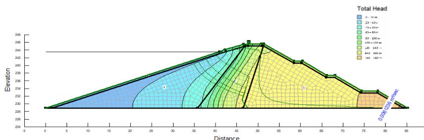
**Figure 7.** Seepage in dam body at Flood water level FWL (+243.98)
