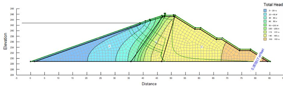
**Figure 8.** Seepage in dam body at Normal water level, NWL (+243.2)
