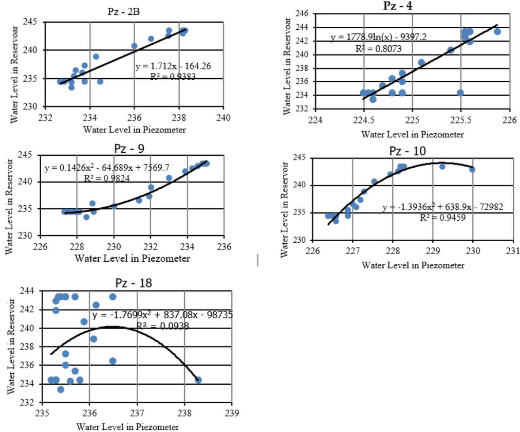
**Figure 5.** Regression value of piezometers to the water level in reservoir
