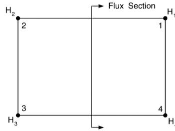
**Figure 1.** Illustration of a flux section across a single element
