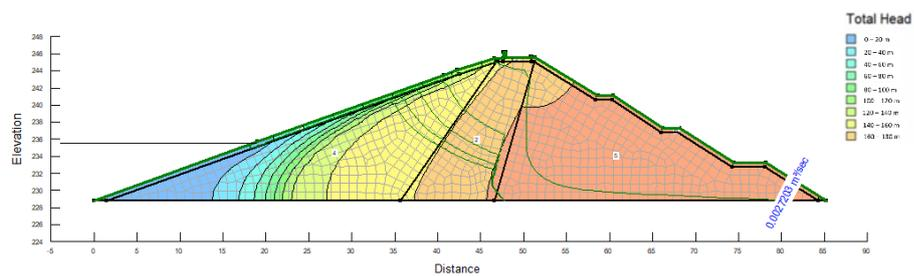
**Figure 9.** Seepage in dam body at Low water level, LWL (+235)
