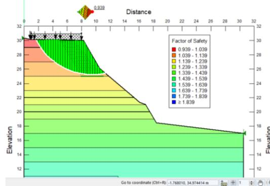
**Figure 3.** Results of Existing Slope Analysis in Normal Conditions
