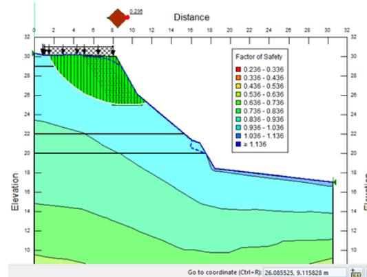
**Figure 4.** Results of Existing Slope Analysis in Moderate Rain Conditions
