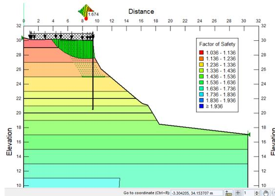
**Figure 5.** Results of Existing Slope Analysis Under Normal Conditions With *Steel Pile Sheet Reinforcement*
