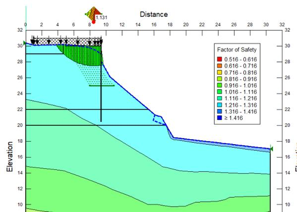
**Figure 6.** Existing Slope Analysis Results In Moderate Rain Conditions With *Steel Pile Sheet Reinforcement*
