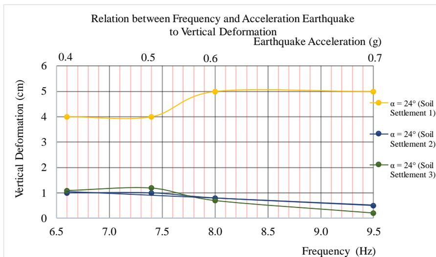
**Figure 6.** Frequency relations and earthquake acceleration of axial deformation at  $\alpha = 24^\circ$
