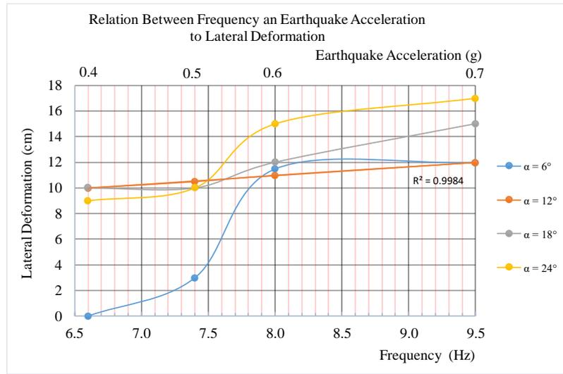
**Figure 5.** Frequency relations and earthquake acceleration against lateral deformation
