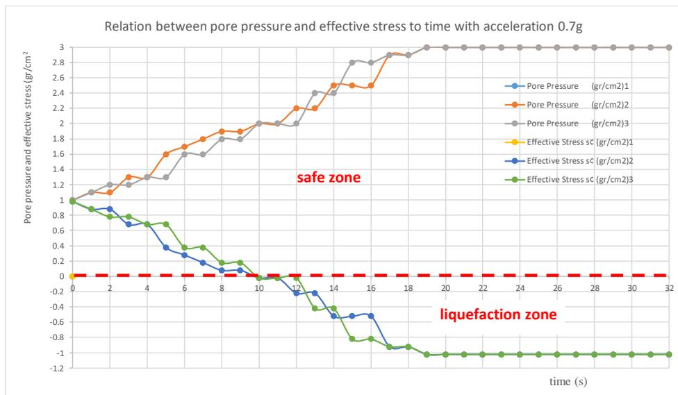
Figure 2. Water pressure pore and effective stress in time with acceleration 0.7 g
