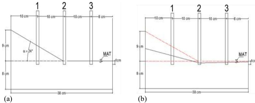
**Figure 3.** Installation piezometer and Shaking Table (a) before and (b) after testing
