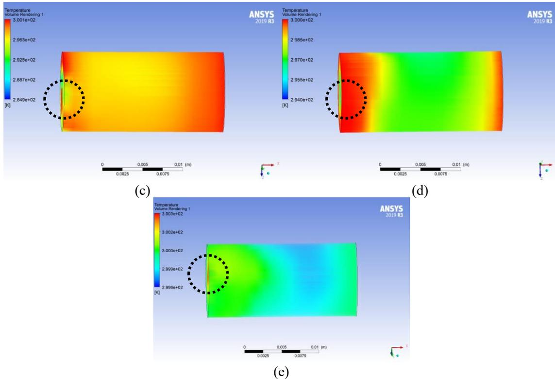
**Figure 4.** The results of the ANSYS simulation of pellet combustion temperature in the variation of the mixture (gelam wood + rice husk): (a). 100% gelam composition, (b). Gelam composition 80%: Rice husk 20%, (c). 60% Gelam Composition: 40% Husk, (d) 50% Gelam Composition: 50% Husk and (e). 100% Husk Composition
