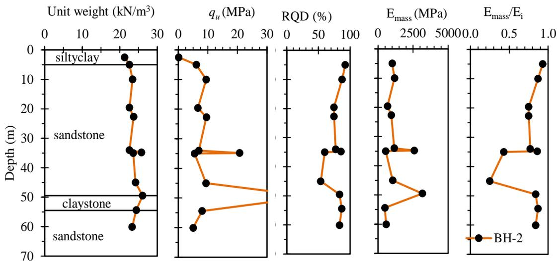
Figure 2. Geotechnical rock properties of BH-2
