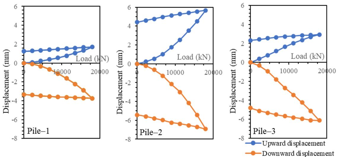
**Figure 4.** Upward and downward displacement obtained from OC tests
