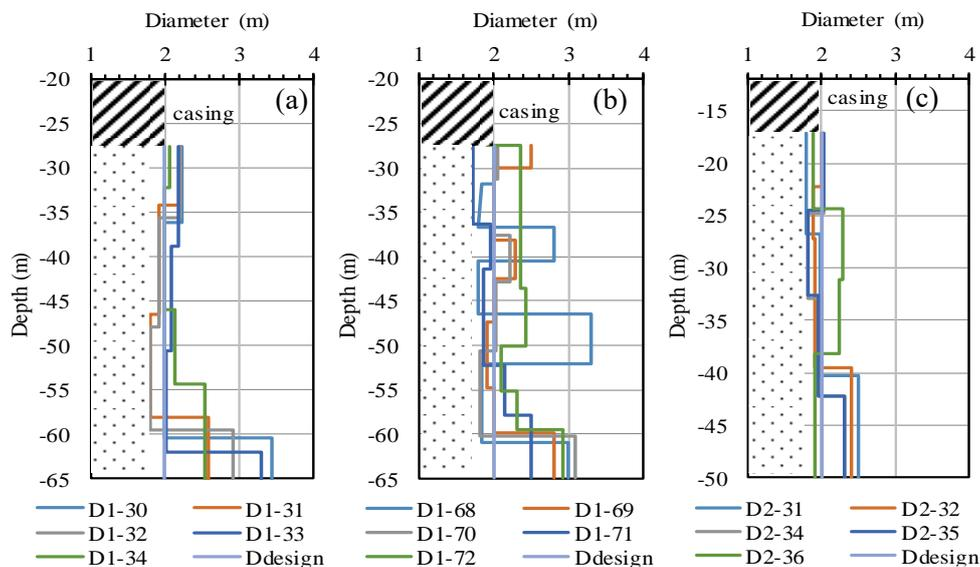
**Figure 5.** Calculated bore diameter (a) Pile Cab 1, (b) Pile Cab 2, and (c) Pile Cab 3.
