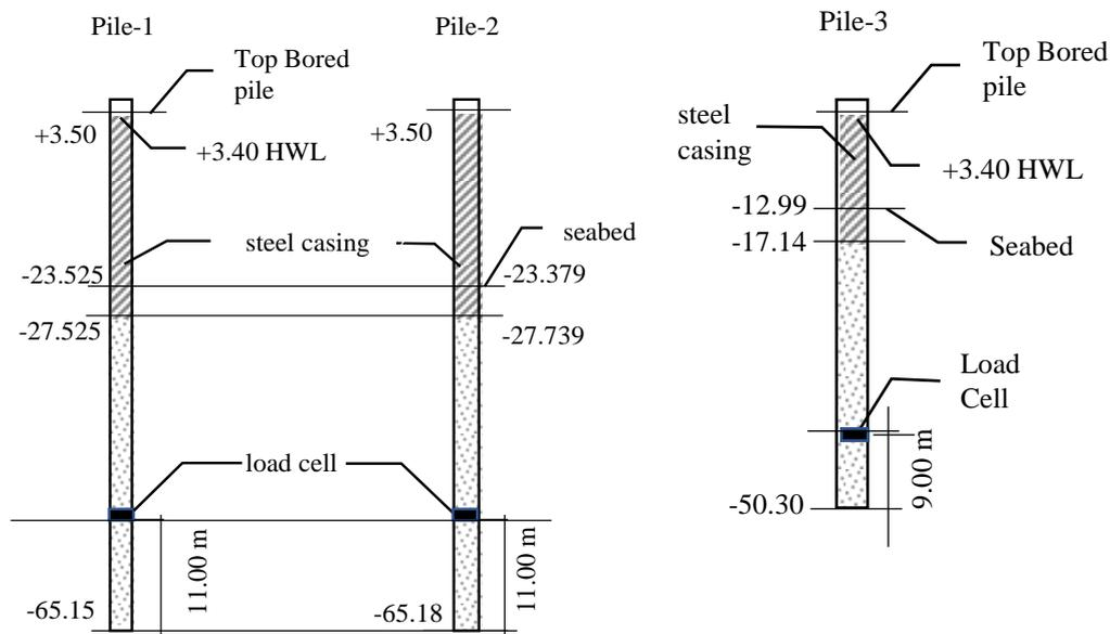
**Figure 3.** Sketches of pile and load cell positions Pile-1, Pile-2, and Pile-3
