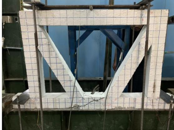
**Figure 3.** Cyclic loading test on the loading frame
