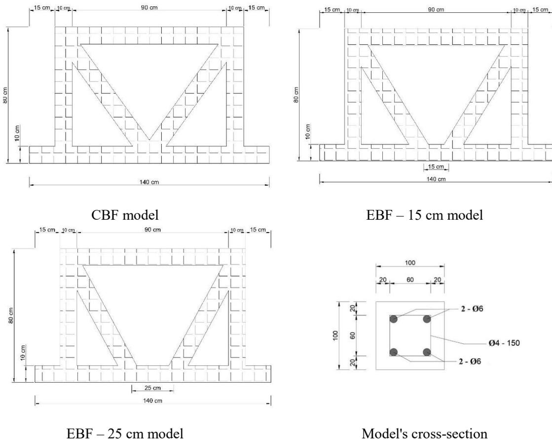
**Figure 1.** Detailed dimensions of CBF and EBF models
